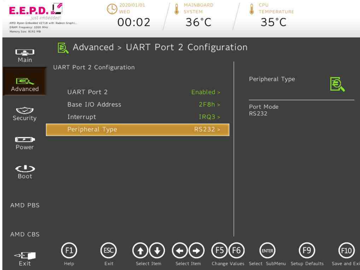
Fig. 73: UART Port 2 Configuration
